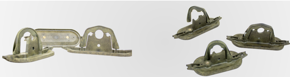
Cryogenic piping brackets injection molded from Torlon 7130 PAI
